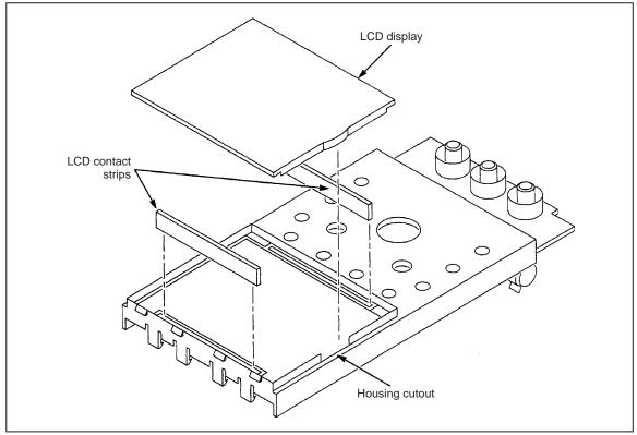
Figure 4. Reassembling the LCD
