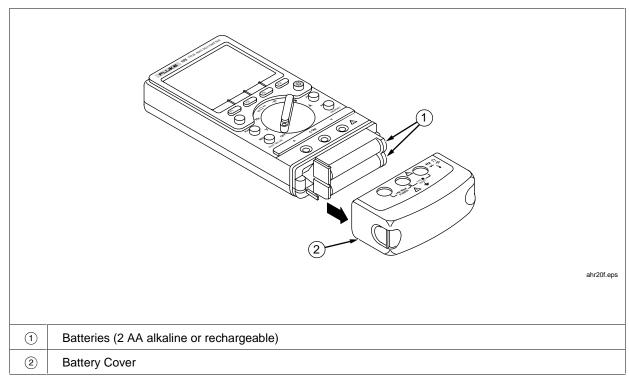
Figure 5. Replacing the Batteries
